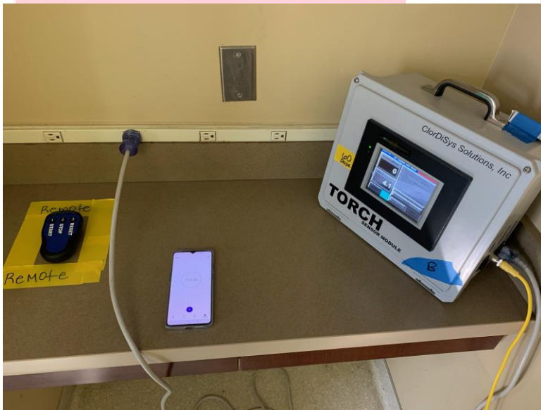
Figure 12 – Start cycle on remote. Start logging on touchscreen.
